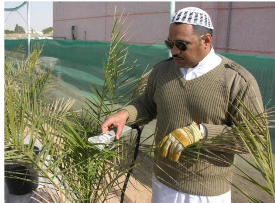
Portable open system LCi to measure gas exchange for photosynthesis
